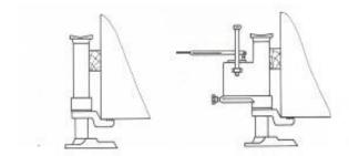
9-If the loading height is insufficient to adhere to the previous instruction, the leg must be used over its entire length.
